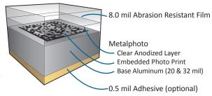
good resistance to most general purpose cleaners, mild acids, oil and water. The SandShield label comes with holes for mechanical attachment or a 5.0 mil high performance adhesive designed to permanently bond to metals and low surface energy (LSE) materials. An optional CARC adhesive is also available.
