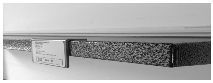
The ArmorerLink® Shelf Label Holder (SLH) kit is utilized in situations where there is insufficient surface area to affix a label measuring W 2.40 in. x H 2.00 in. (6.09 cm x 5.08 cm). The SLH has double-sided tape on the top and bottom surface of the base for multiple mounting options. The SLH is reusable by replacing the double-sided tape. For permanent installations, the SLH can be mounted using mechanical fasteners.
